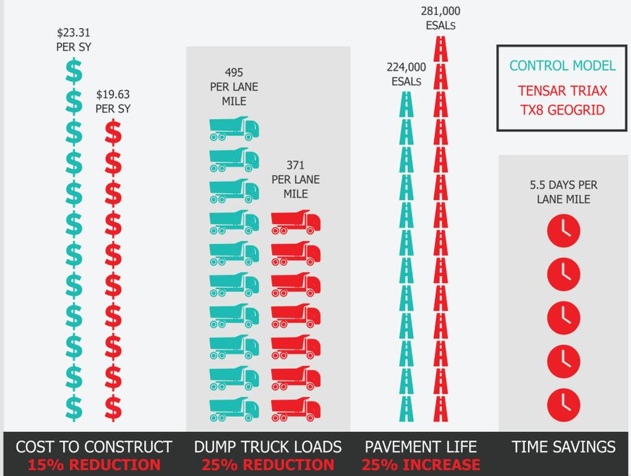
Using Tensar TriAx Geogrids can offer **significant initial construction cost savings** of around 15%. The number of **dump trucks** traveling over existing infrastructure to service a project can be reduced by 25%. The **pavement life** can be improved from 19-25%. And the amount of **time to construct** a project can be significantly decreased by approximately 5 days per lane mile.
