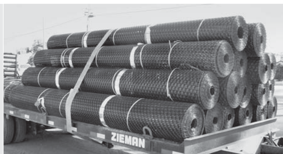
Image 1 Storing the Tensar TriAx Geogrid rolls (horizontally).
