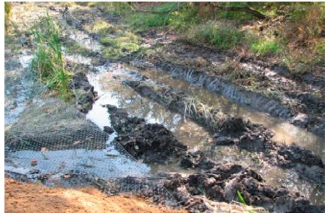
*The subgrade consisted of saturated silty lake sediments with very low shear strength.*
