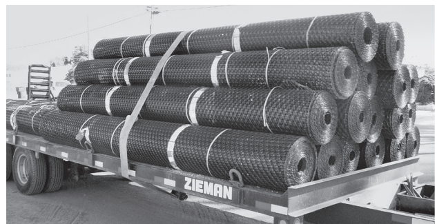
Storing the Tensar Geogrid rolls horizontally.
