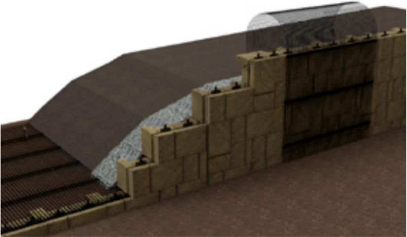
Typically, loose lifts of the reinforced fill shall not exceed 6 in. where hand-operated compaction equipment is used or 10 in. where heavy compaction equipment is used. These thicknesses may vary depending on the approved project-specific soil types used. Compact fill to a minimum of 95% of the maximum dry density, or in accordance with ASTM D-698 (Standard Effort Proctor Test).
