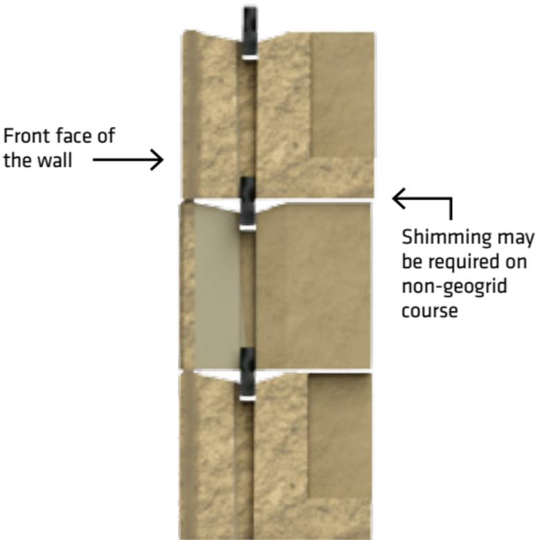
If the design dictates the need for a geogrid at a particular elevation, install the Tensar® Geogrid with the teeth of the Olympia Connectors penetrating through the geogrid apertures. The pin should never be utilized to connect the geogrid to the facing units.
