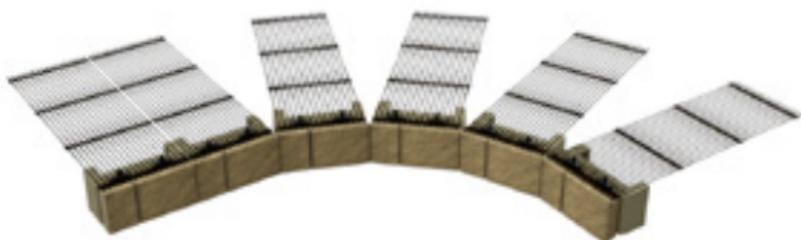
**NOTE:** On tight curves, Tensar<sup>®</sup> Geogrid may be cut lengthwise to the width of the Olympia Units to ensure the transverse bar engages both connectors
