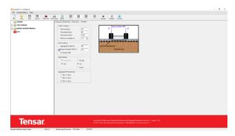
The Subgrade Stabilization module allows the user to determine MSL thickness over a soft subgrade to pass a proof roll or reach the design traffic level.
