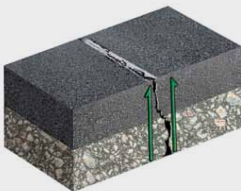
FIGURE 1: Cracks migrate toward surface in an unreinforced overlay.
