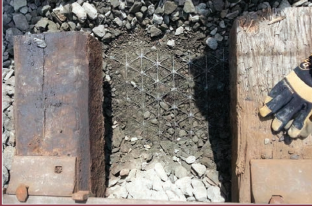
IMAGE A: TriAx TX190L Geogrid was in good condition with no damage observed while continuing to support ballast near the surface.
