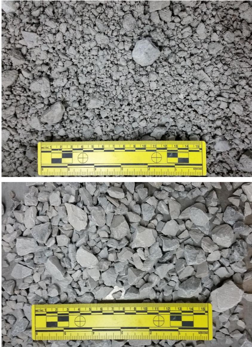
**Figure 11. (top) Full gradation sample and (bottom) gravel retained on No. 4 sieve after washing and oven-drying for the crushed aggregate base material.**
