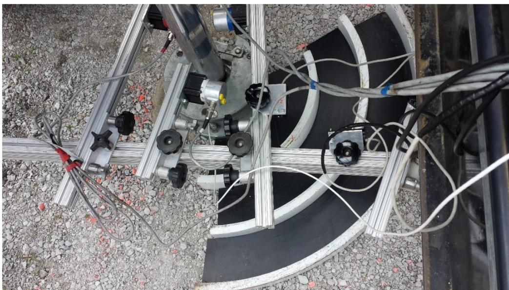
**Figure 3. APLT test setup with deformation measurements obtained at  $2r$ ,  $3r$ , and  $4r$  from the plate center axis.**
