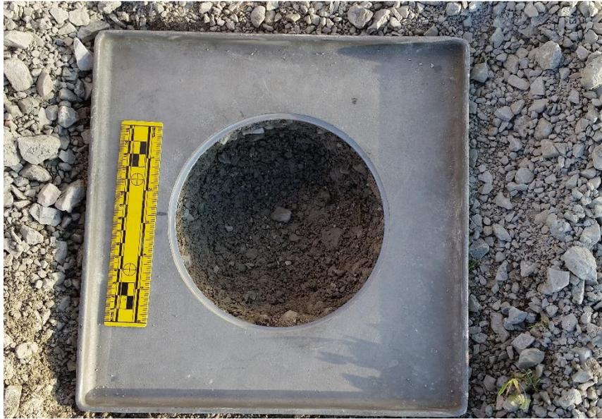
**Figure 5. Picture of an excavated hole ready for sand cone testing.**
