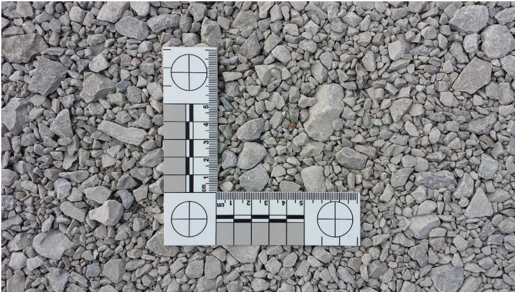
**Figure 8. Aggregate base layer surface at the time of testing.**
