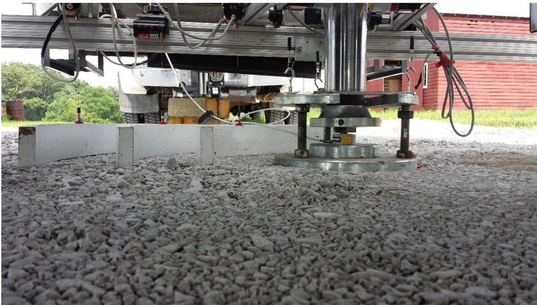
**Figure 9. APLT setup showing 12 in. diameter plate and the 2r, 3r, and 4r deflection basis measurement rings.**
