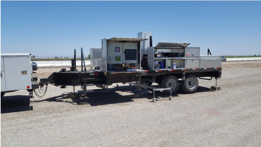
**Figure 1. APLT test system used on I-8 project.**
