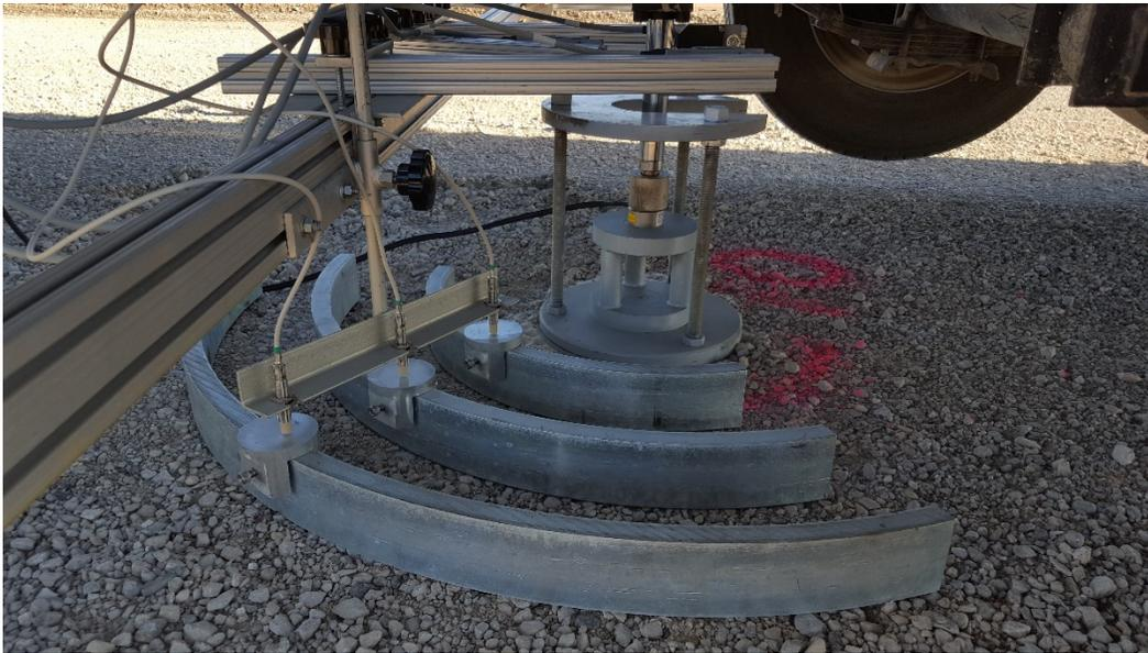
**Figure 4. APLT test setup with deformation measurements obtained at  $2r$  and  $3r$  from the plate center axis.**
