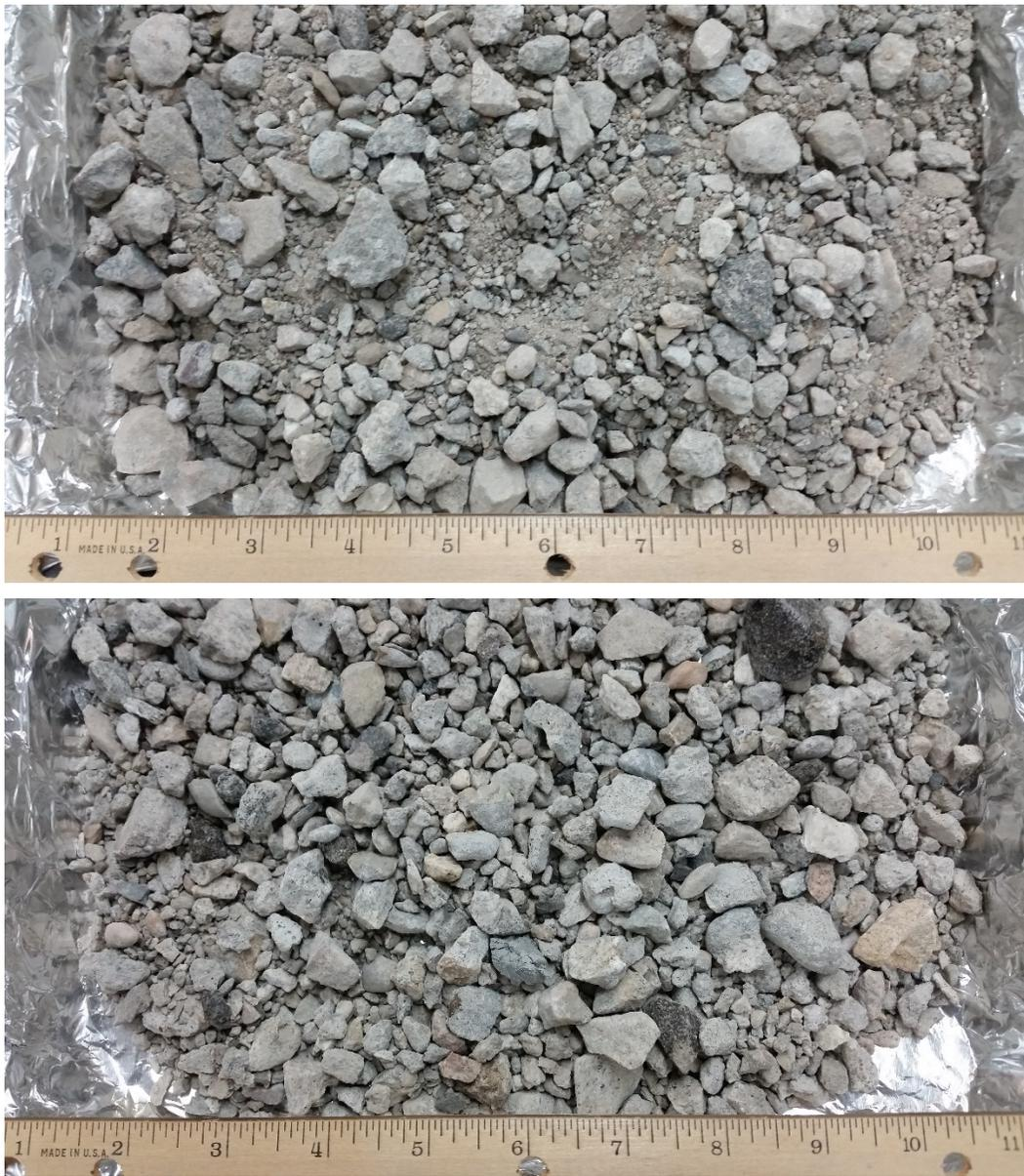
**Figure 11. (top) Full recycled concrete aggregate (RCA) gradation sample and (bottom) material retained on No. 4 sieve after washing and oven-drying (May 10, 2016 sample).**
