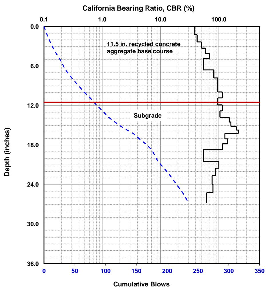
Dynamic Cone Penetrometer (DCP) Test Results
