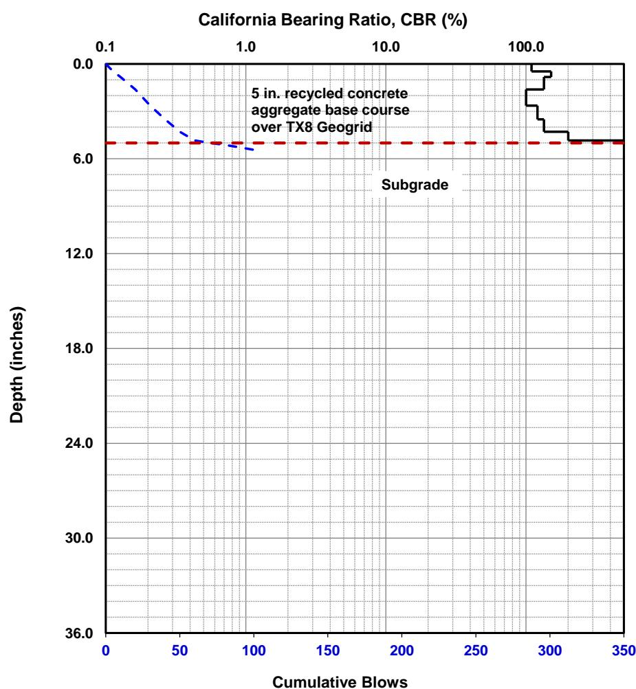
Dynamic Cone Penetrometer (DCP) Test Results
