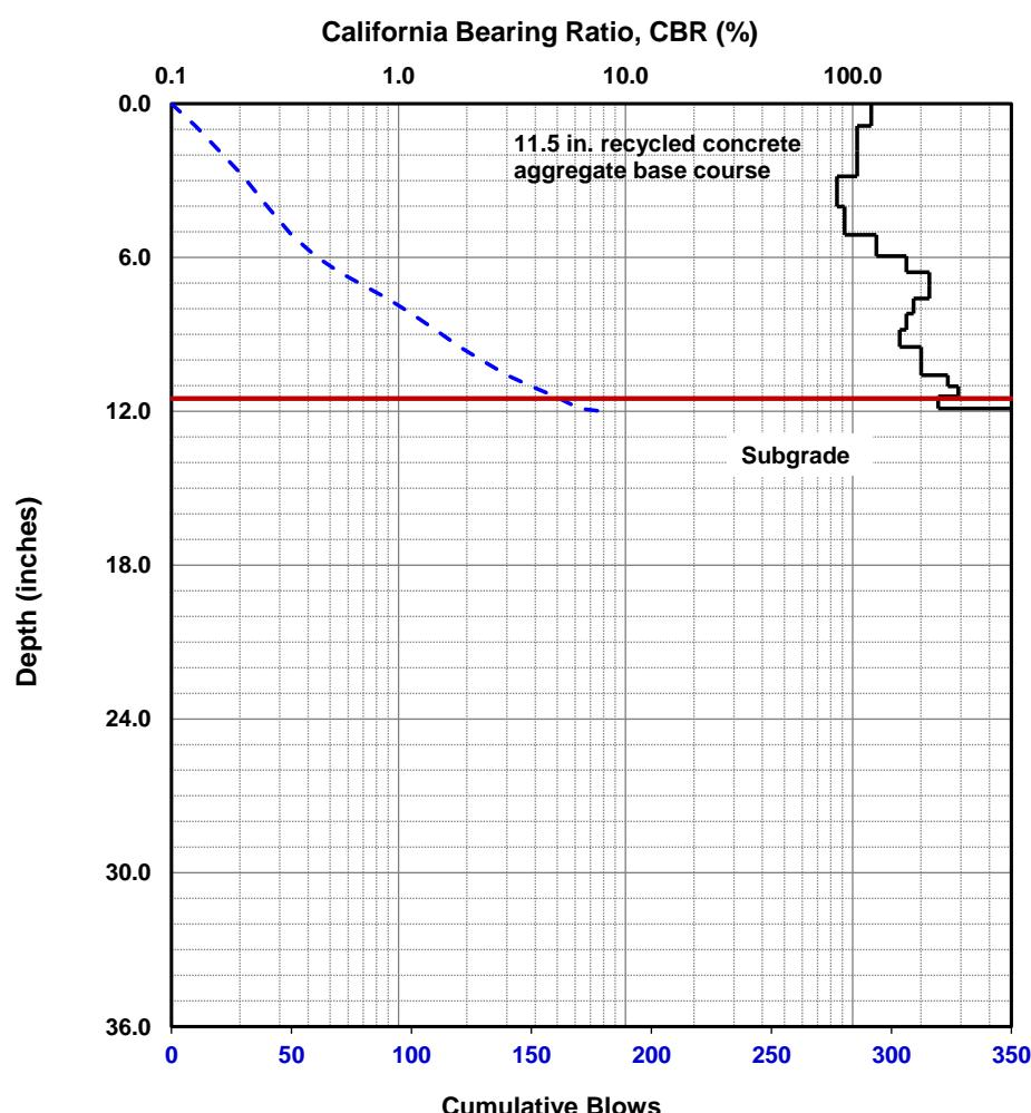
**Dynamic Cone Penetrometer (DCP) Test Results**
