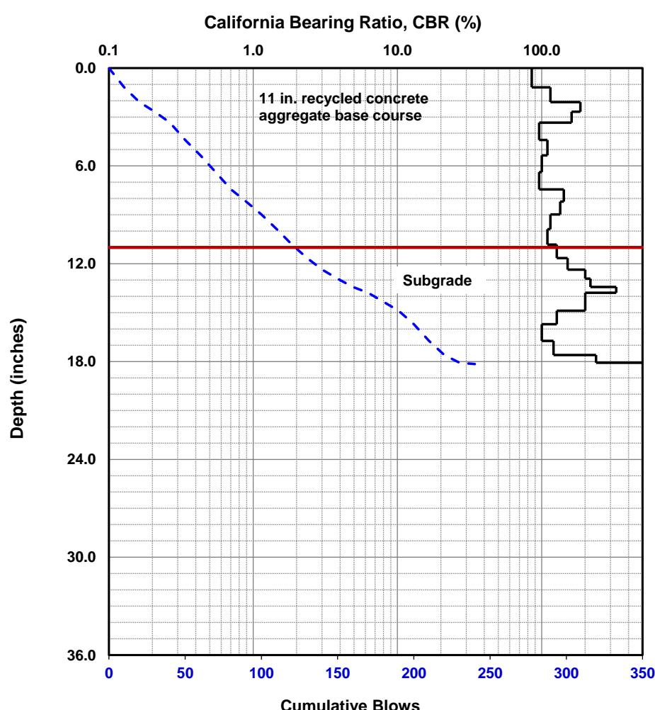
Dynamic Cone Penetrometer (DCP) Test Results
