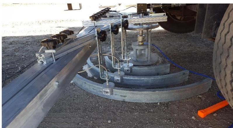
In-situ Resilient Modulus [Mr]: Cyclic Loading, Composite, Stress-Dependent
