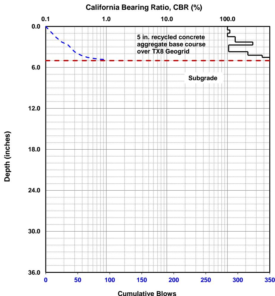
Dynamic Cone Penetrometer (DCP) Test Results
