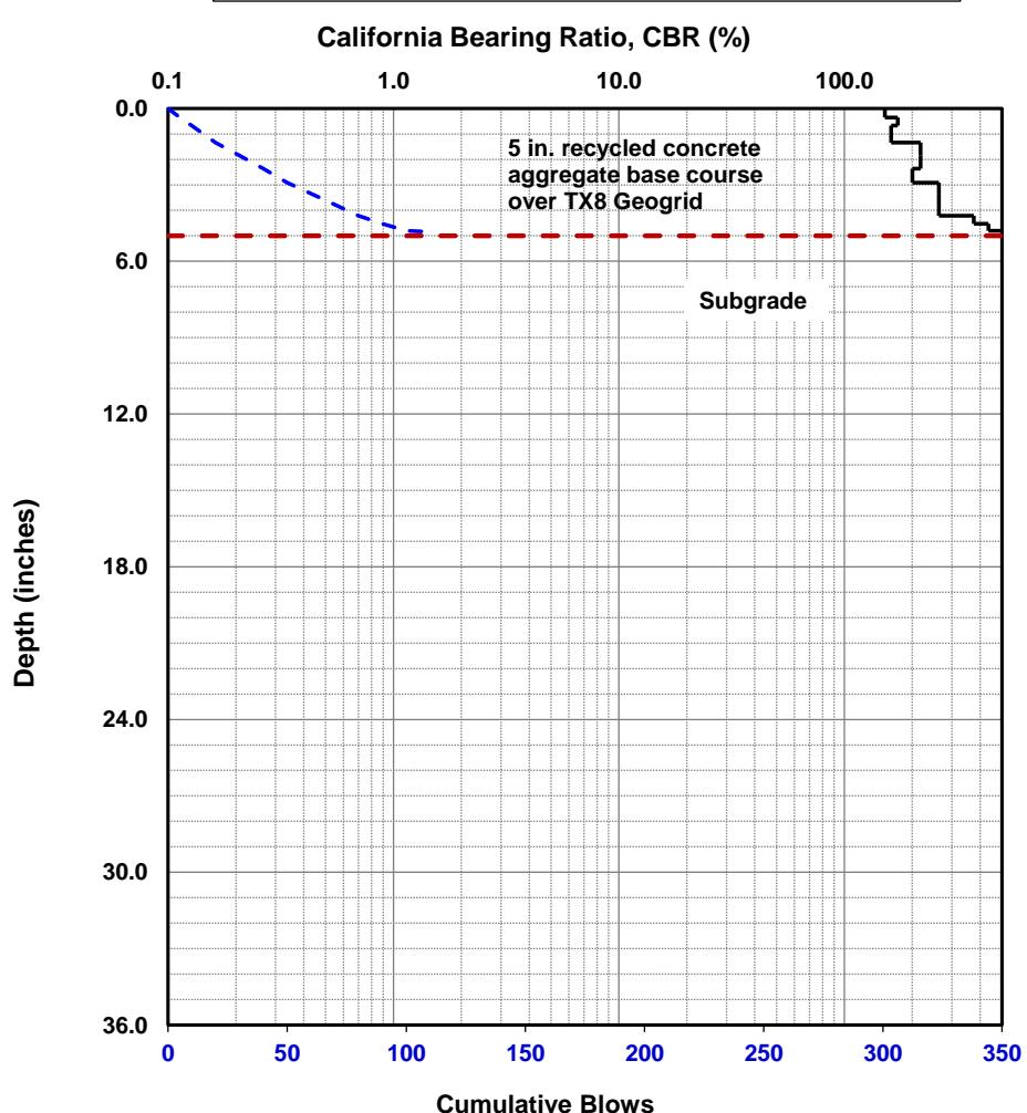
Dynamic Cone Penetrometer (DCP) Test Results
