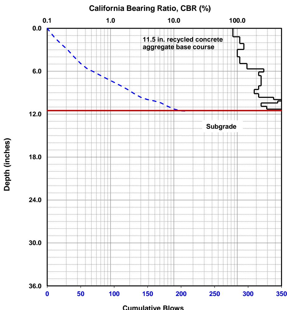
Dynamic Cone Penetrometer (DCP) Test Results
