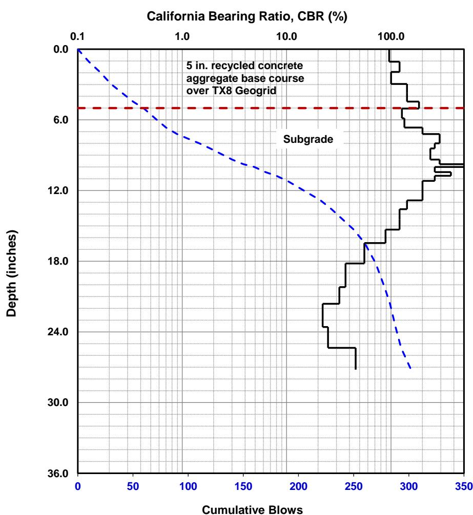
Dynamic Cone Penetrometer (DCP) Test Results
