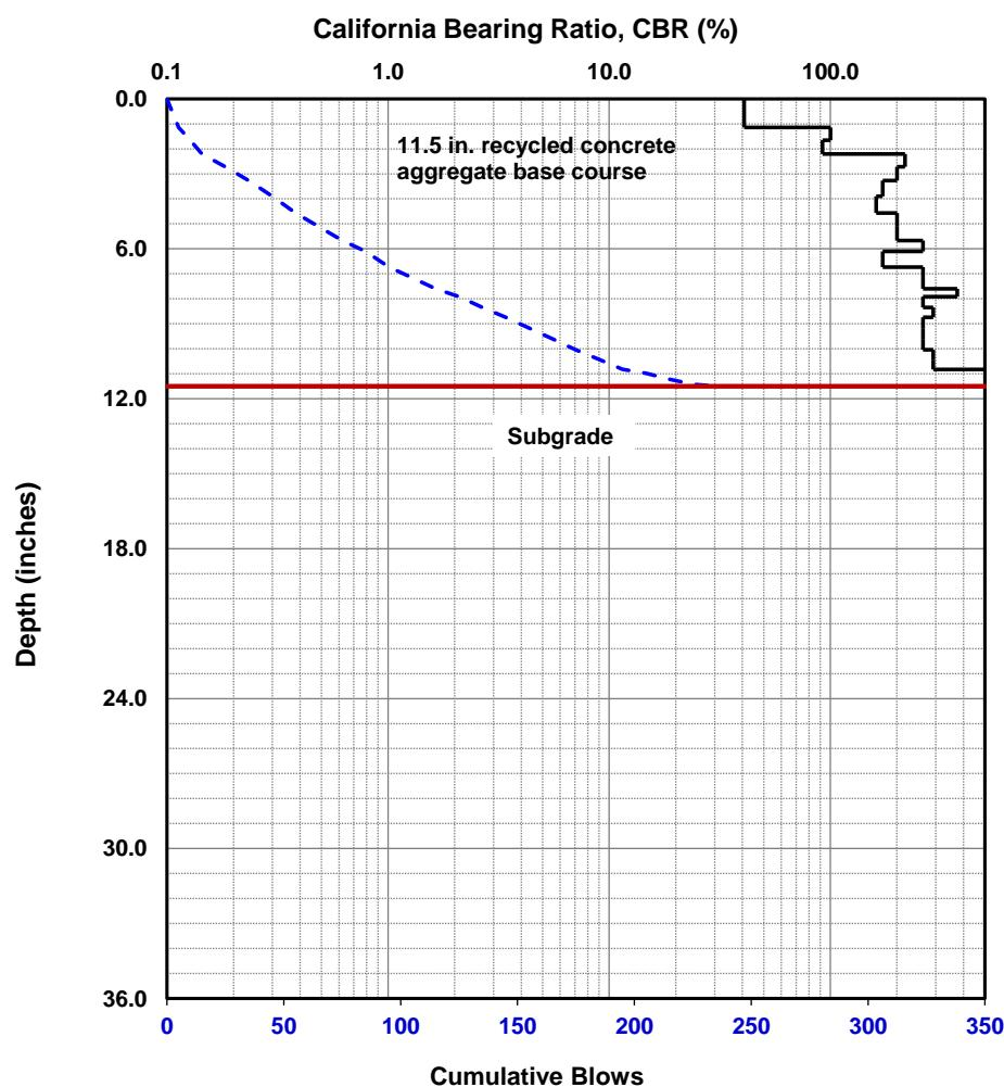
Dynamic Cone Penetrometer (DCP) Test Results
