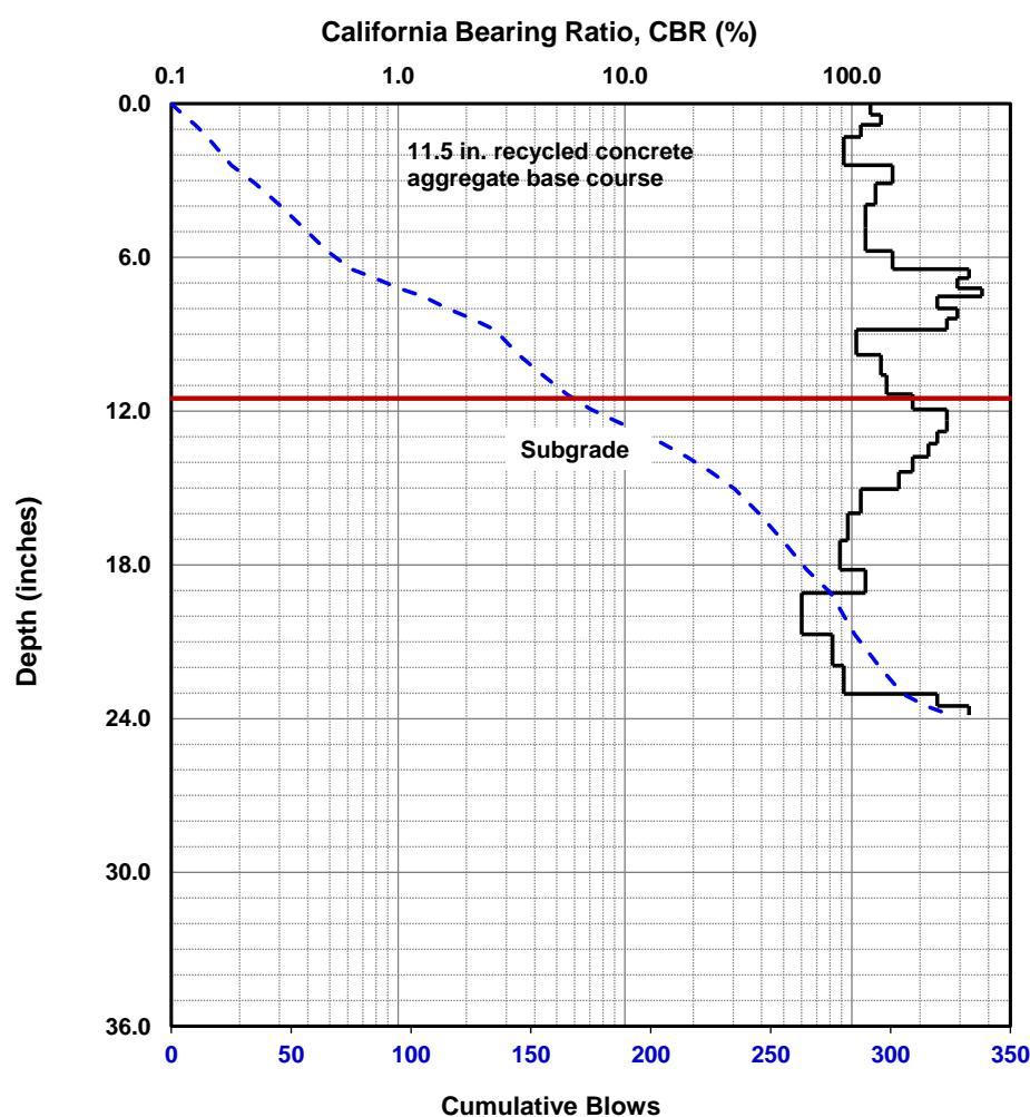
**Dynamic Cone Penetrometer (DCP) Test Results**
