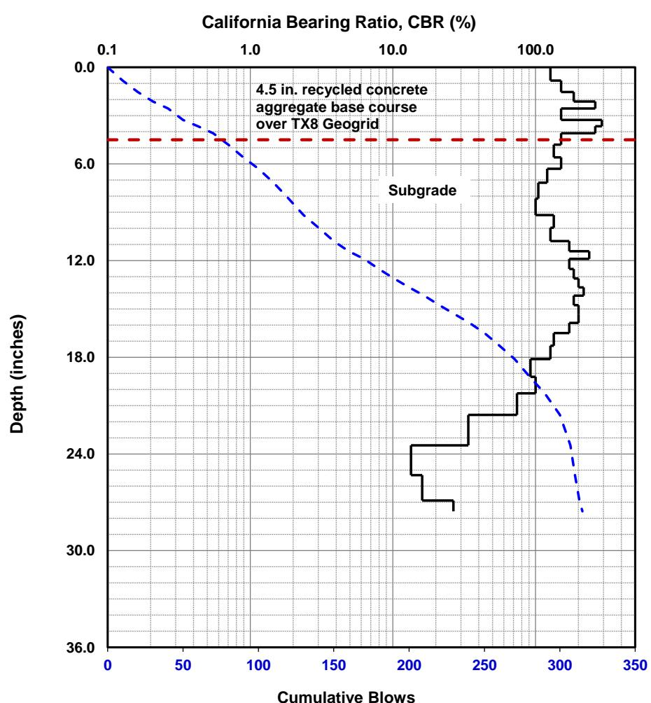
Dynamic Cone Penetrometer (DCP) Test Results
