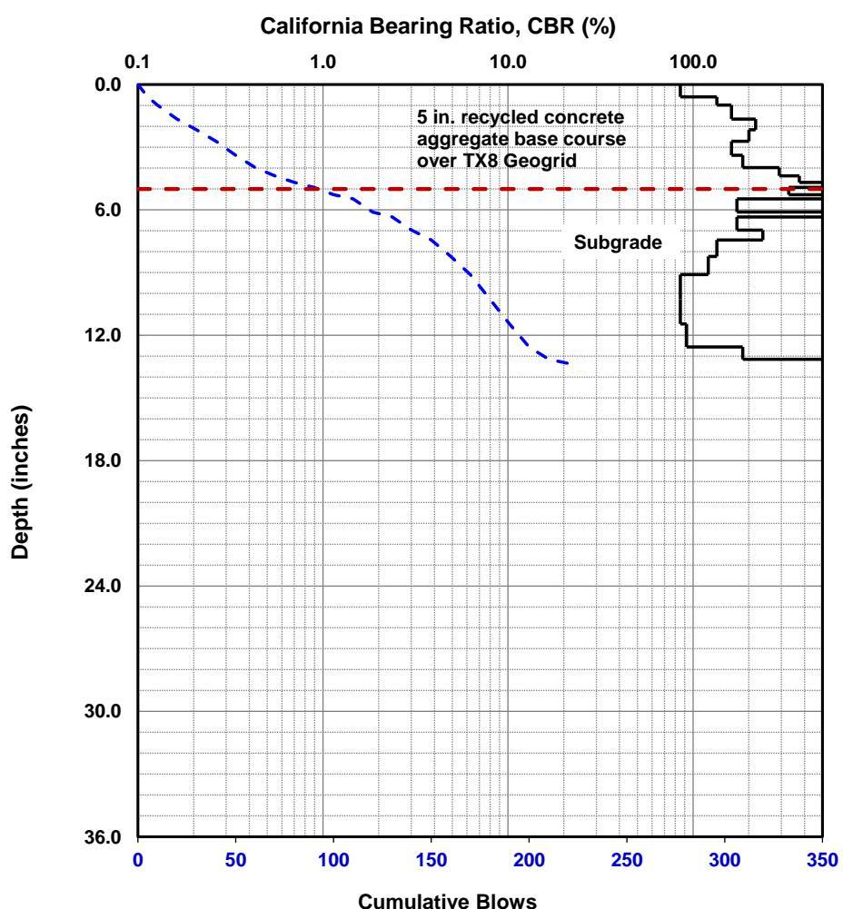
**Dynamic Cone Penetrometer (DCP) Test Results**
