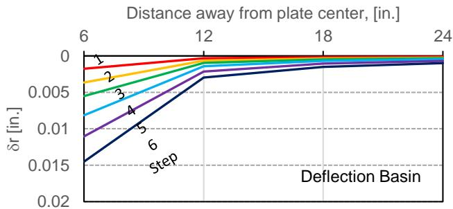
In-situ Resilient Modulus [Mr]: Cyclic Loading, Layered Analysis, Stress-Dependent
