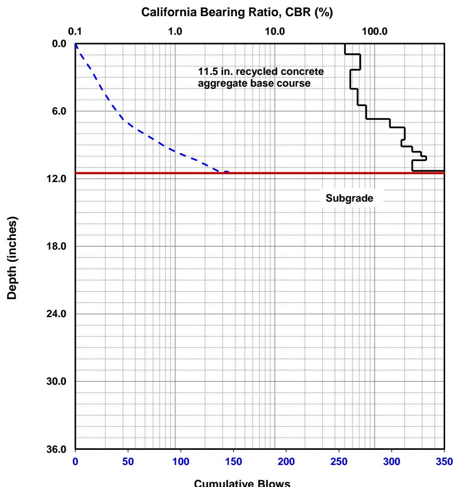
Dynamic Cone Penetrometer (DCP) Test Results
