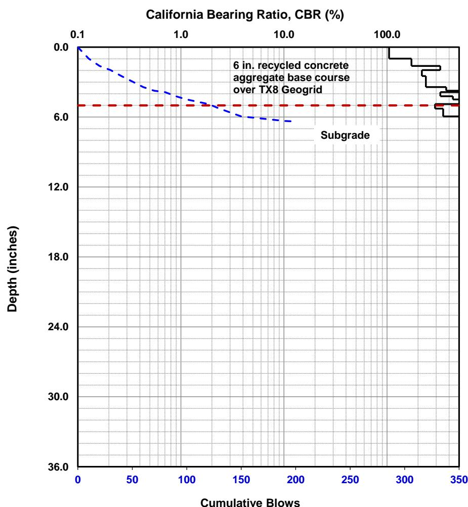
**Dynamic Cone Penetrometer (DCP) Test Results**
