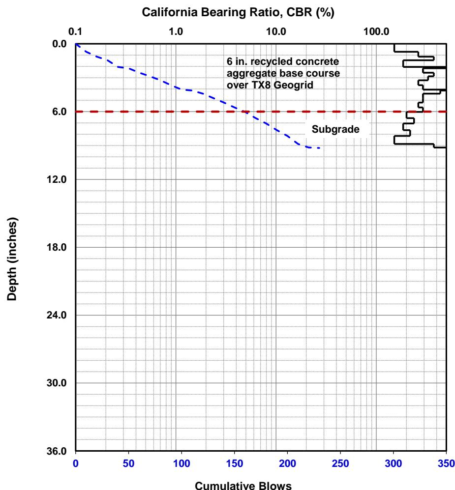
**Dynamic Cone Penetrometer (DCP) Test Results**
