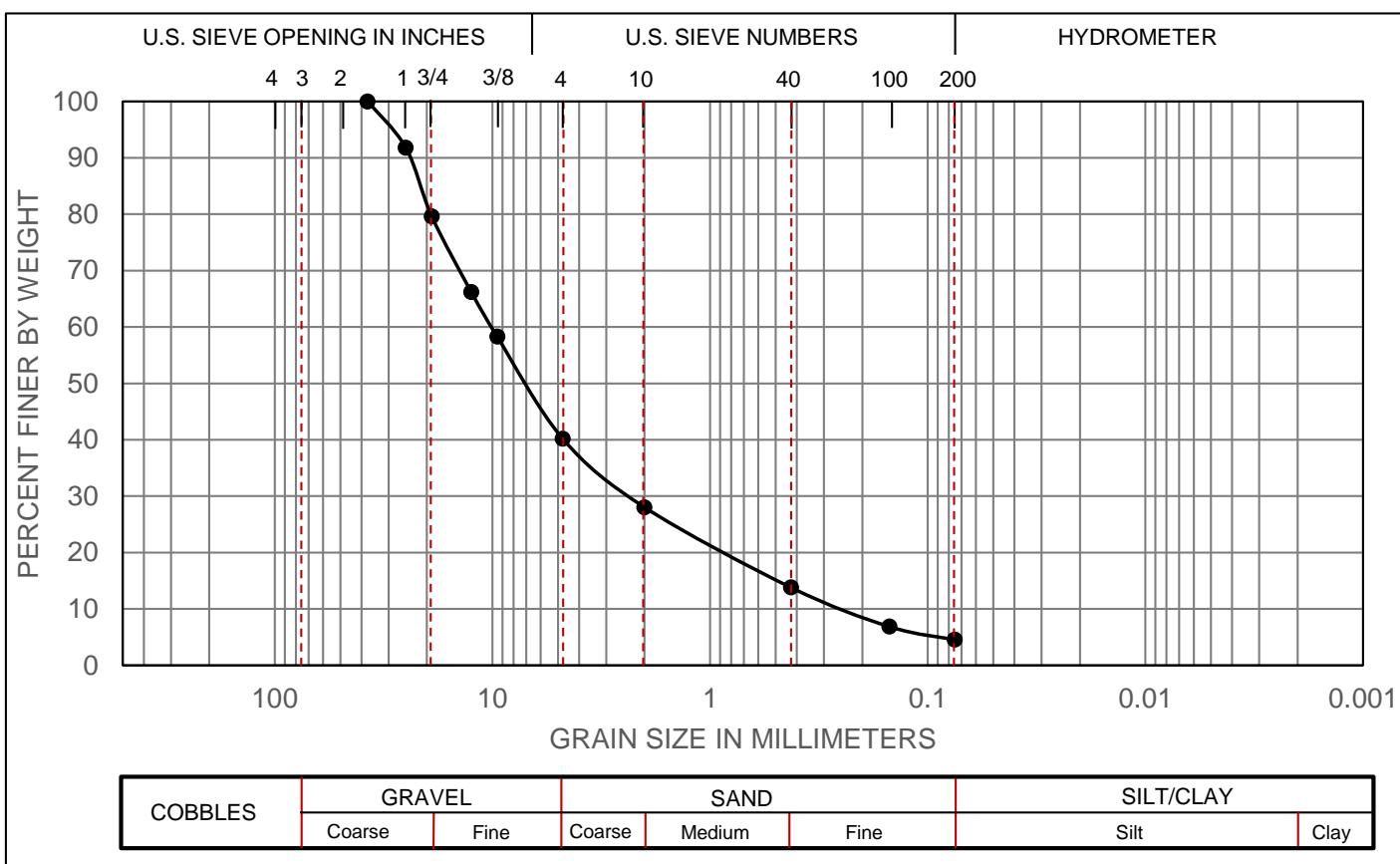
**MATERIAL:** Recycled crushed aggregate (natural moisture content = 5.2%)
