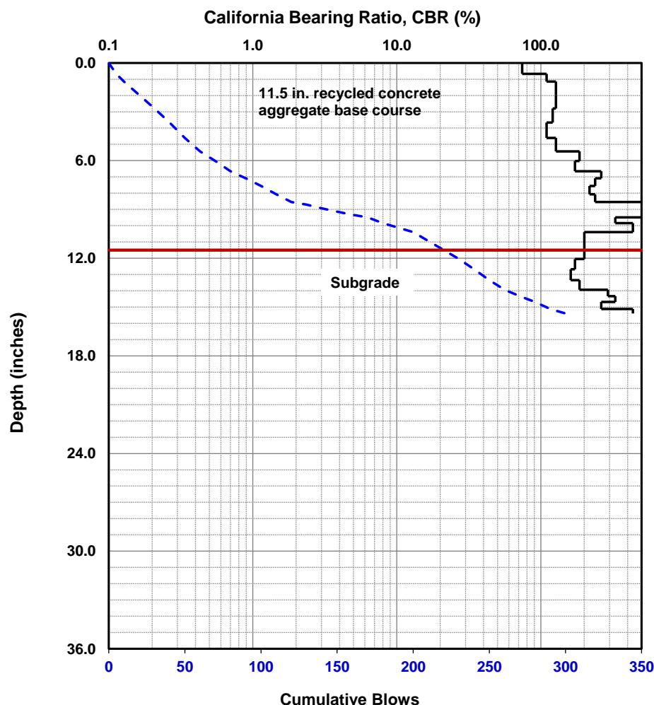
Dynamic Cone Penetrometer (DCP) Test Results
