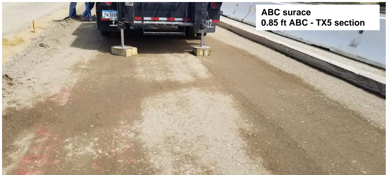
Test point locations on ABC surace 0.85 ft ABC - TX5 section
