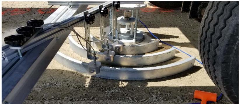
In-situ Resilient Modulus [Mr]: Cyclic Loading, Composite, Stress-Dependent
