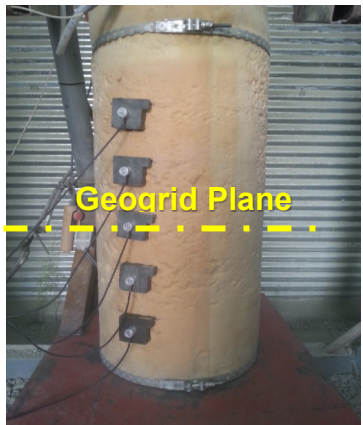
Figure 3. Large scale triaxial compression test on 1.0 m high and 0.5 m diameter specimen.
