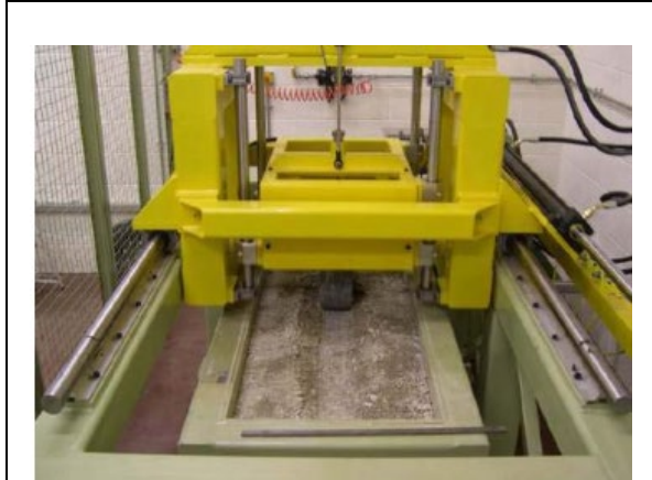
Figure 1. The Tensar Small Scale Trafficking device in service, with pressure applied by the tire of ~600 kPa equivalent to that of conventionally loaded truck tire.
