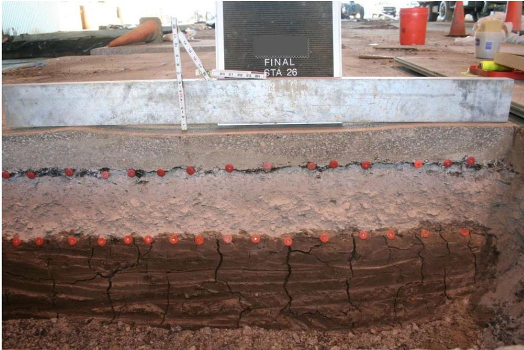
Figure 37. Item 1 post-traffic layer thicknesses.
