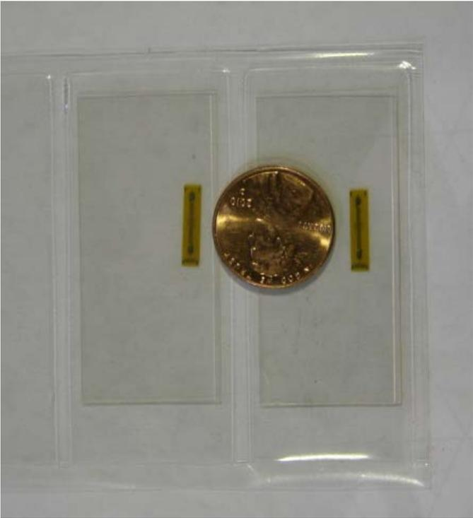
Figure 11. Strain gauges installed on the geogrid.
