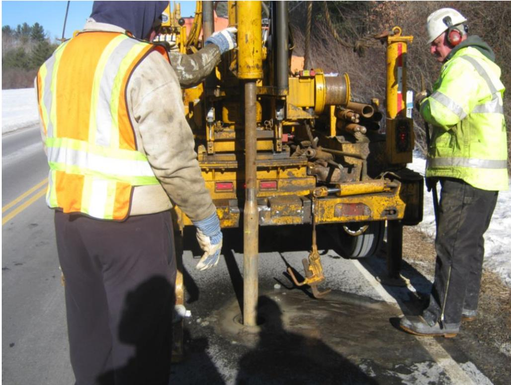
Figure 4. Cored asphalt concrete at location FT5.
