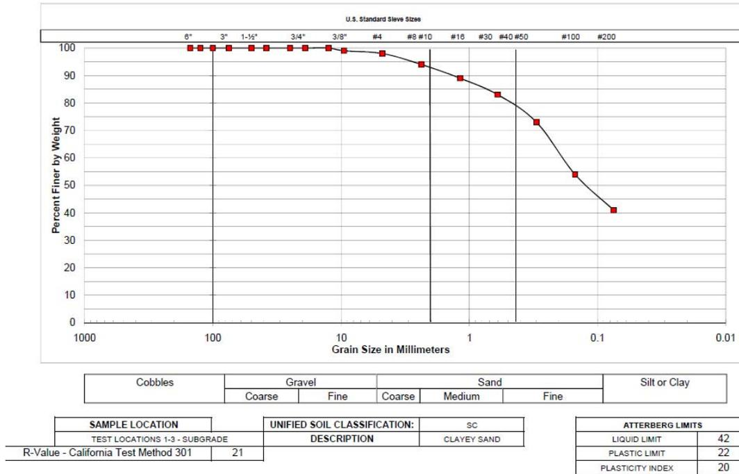
Figure 2 – Subgrade Soil Testing Results
