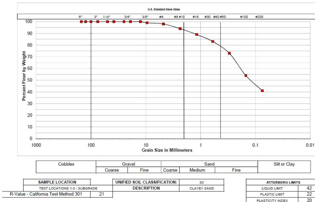
Figure 2 – Subgrade Soil Testing Results
