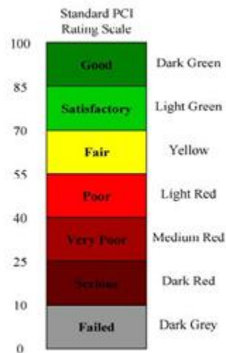
Figure 2. ASTM D-6433 scale for PCI ratings.
