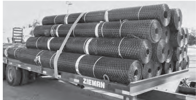
IMAGE 1: Storing the Tensar TriAx Geogrid rolls (horizontally).
