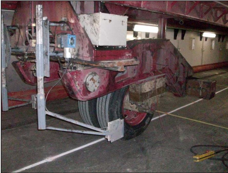
Photo 6. Dual-wheel single axle used to traffic Item 4.
