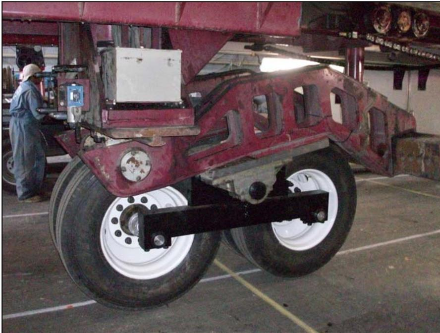
Photo 7. Dual-wheel tandem axle used to traffic Items 1, 2 and 5.
