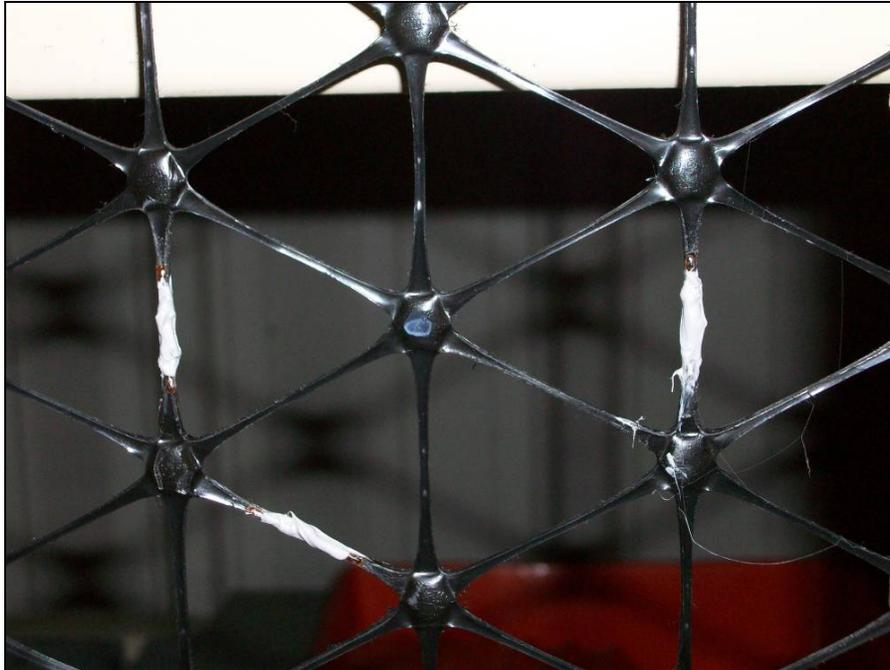
Photo 3. Geogrid strain gauges on TriAx geogrid product prior to placing epoxy protective layer.
