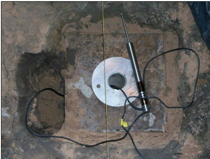
Photo 5. SDD housing prior to placement of LVDT.
