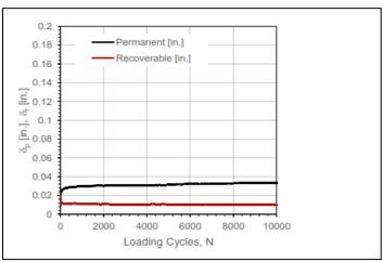
The plots above show the permanent and recoverable deformation measured. The control section showed about 3 times more permanent deformation than the TriAX section over the 10,000 cycles.
