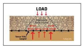
the potential for contamination of the aggregate base with the subgrade soil. The geogrid and aggregate base together create a mechanically stabilized layer (MSL). The MSL provides a resilient layer that minimizes the potential for differential movements of the concrete surface that initiate faulting and corner breaks.
