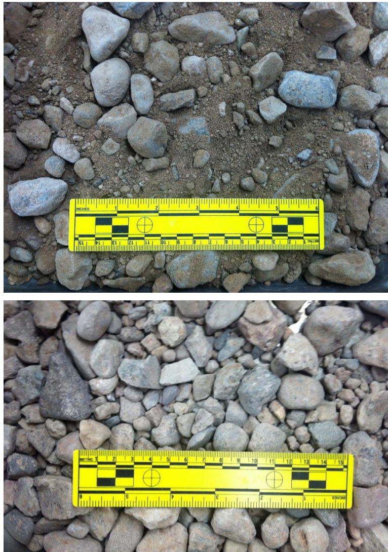
Figure 11. (top) Full gradation sample and (bottom) aggregate base course retained on No. 4 sieve after washing and oven-drying (April 17, 2015 sample).
