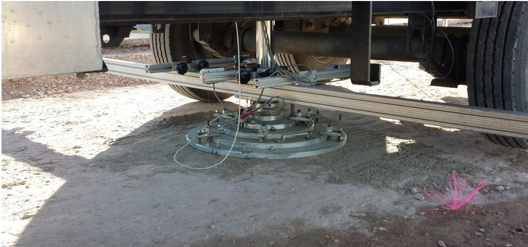
Figure 5. APLT test setup with 30 in. diameter plate for AASHTO T222 static plate load test (note: wheels not in contact with ground during testing).
