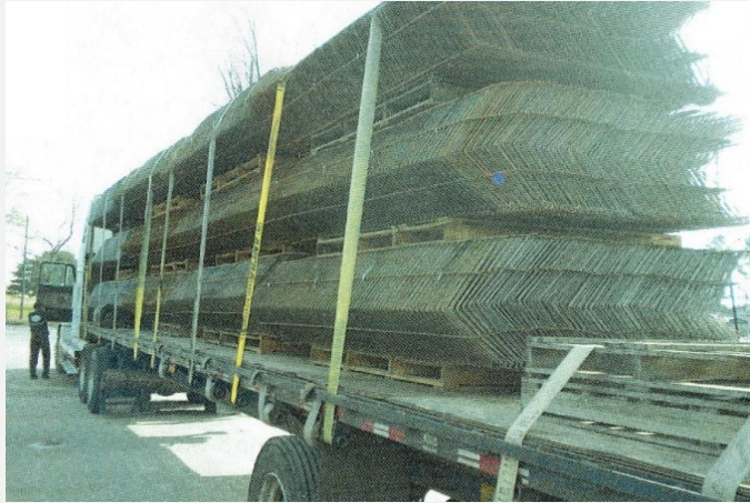
Up to 1500 baskets/truck 21,000 SF of wall face
