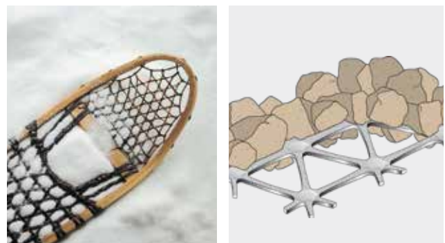
FIGURE 4 As a snowshoe distributes load over soft snow, Tensar TriAx Geogrid confines aggregate to better distribute in-service loads over soft subgrades.
