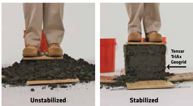
FIGURE 1 The lateral confinement of aggregate reinforcement with Tensar TriAx Geogrid is shown through the box of rocks demonstration.
