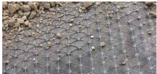
Tensar TriAx Geogrids, designed to interlock and confine aggregate particles to create a mechanically stabilized layer with improved bearing capacity.
