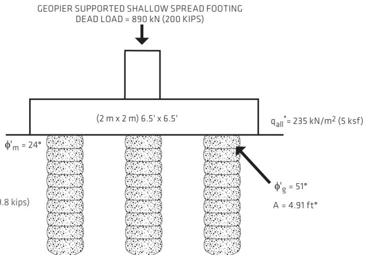
\*  $q_{\text{all}}$  is greater for Geopier supported footings than for conventional footings because of the increased shearing strength afforded by the Geopier elements.
