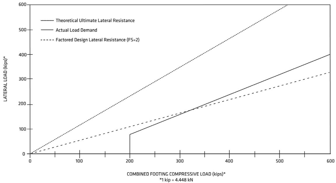
Note: Figure neglects additional lateral load resistance provided by steel uplift bars.
