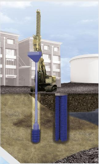
The Impact system doesn't generate spoils, so there are fewer equipment and transportation needs, which also provides a cost benefit.
