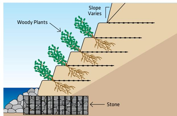
Cross section view of VRSS showing marine mattresses as toe protection and foundation support at the submerged toe of the reinforced slope.
