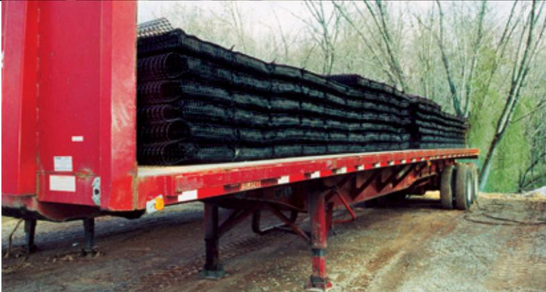
› Manufactured from durable polymers, these geogrids resist chemical, biological and environmental degradation to ensure long-term structural integrity and service life.
