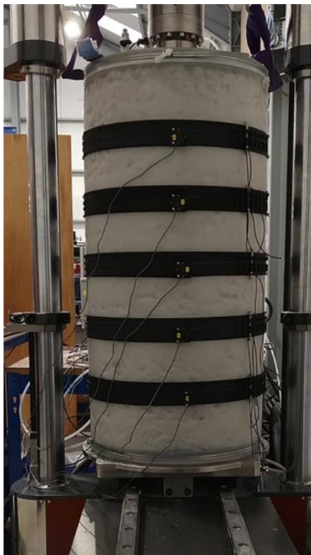
Figure 2 – 1.0m x 0.5m large triaxial test rig
