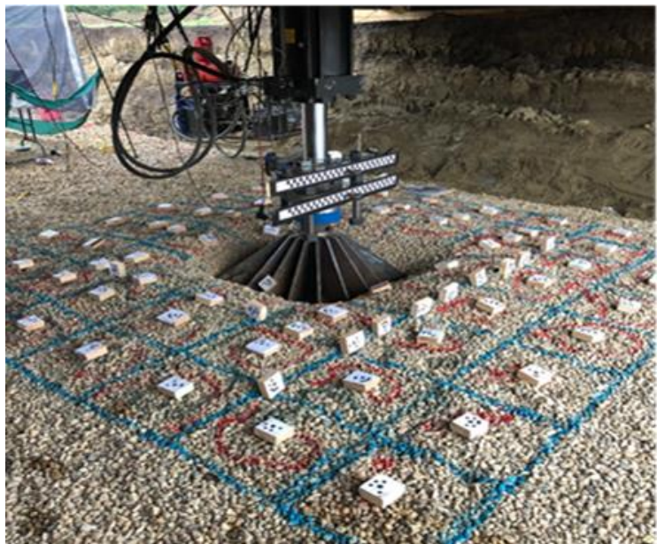
Figure 6 - completed test at Saskatchewan showing bearing capacity failure of the 1.0m 2 steel plate positioned under the counterweight bridge shown in
