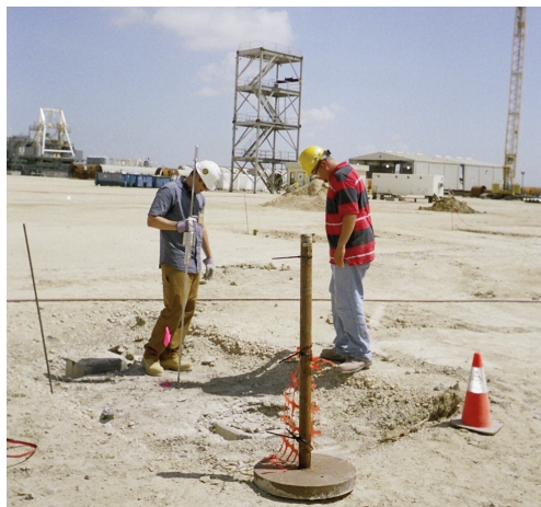
In 2007, DCP testing was conducted at the site to determine section stability.
