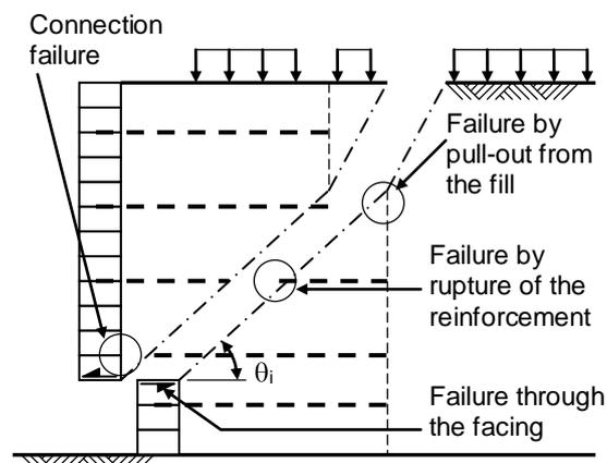
Figure 4. Likely mode of failure of two wedges
