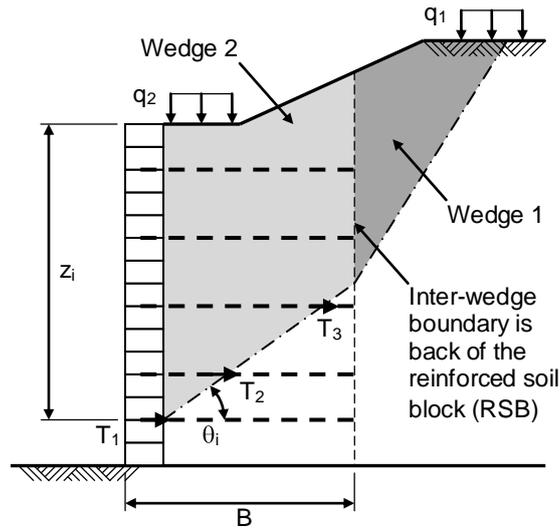
Figure 1. Basis of the two-part wedge method
