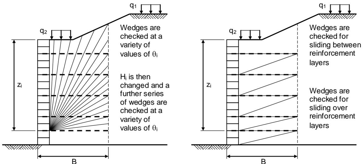
Figure 2. Search routines used with two-part wedge method
